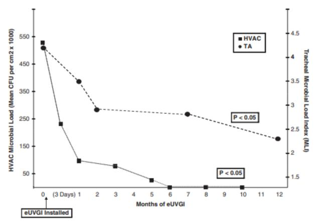
*Figure II-3 Ultraviolet germicidal irradiation (UVGI) decreased the microbial load of the heating ventilation and air conditioning system (HVAC).* [10]
