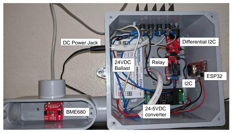
Figure B-3 Inside Prototype Hardware [30]
