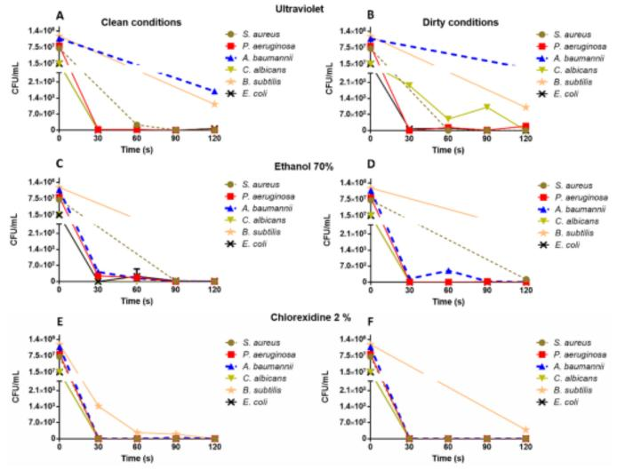
Figure II-2 UV-C disinfection in clean and dirty conditions at different exposure times [12]
