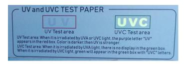
Figure IX-1 Low-pressure Mercury Vapor UV-C lamp Indicator [27]
