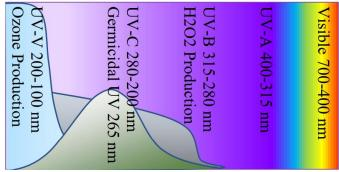
Figure II-1 UV light spectrum [3].
