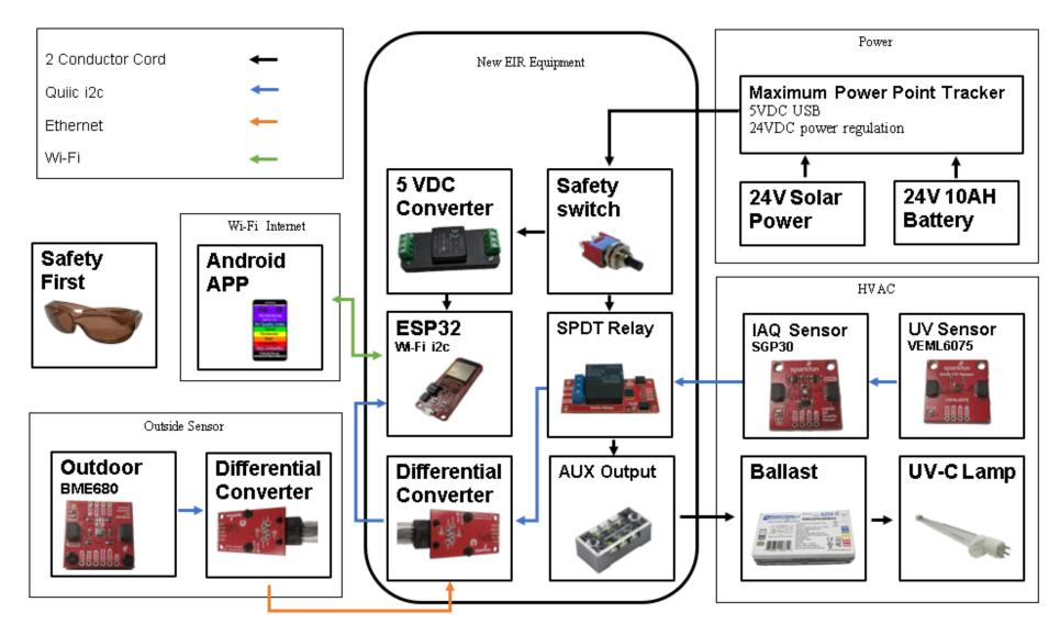
Figure B -3 New-EIR Hardware Connections[30]
