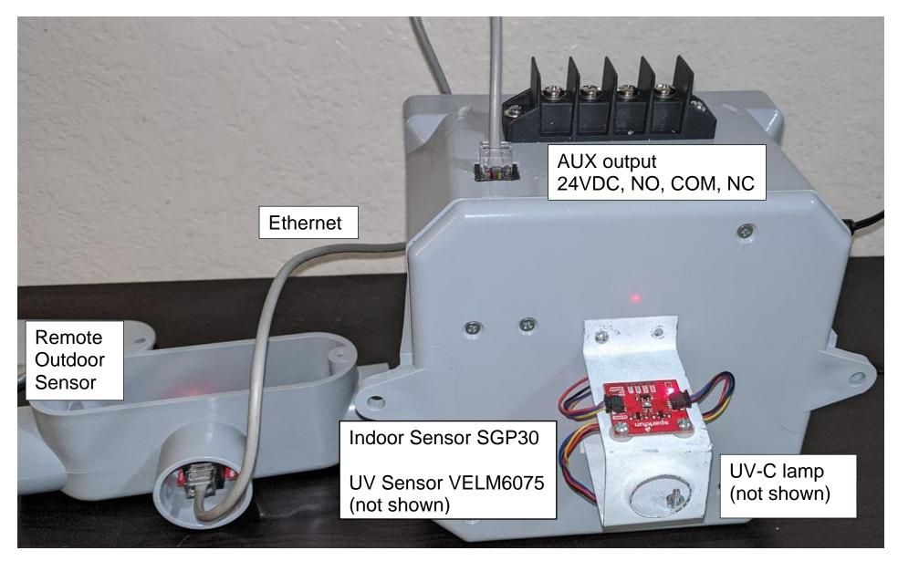
Figure B-4 Outside Prototype Hardware [30]
