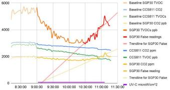
Figure IX-3 TVOCs lower by UV-C [27]
